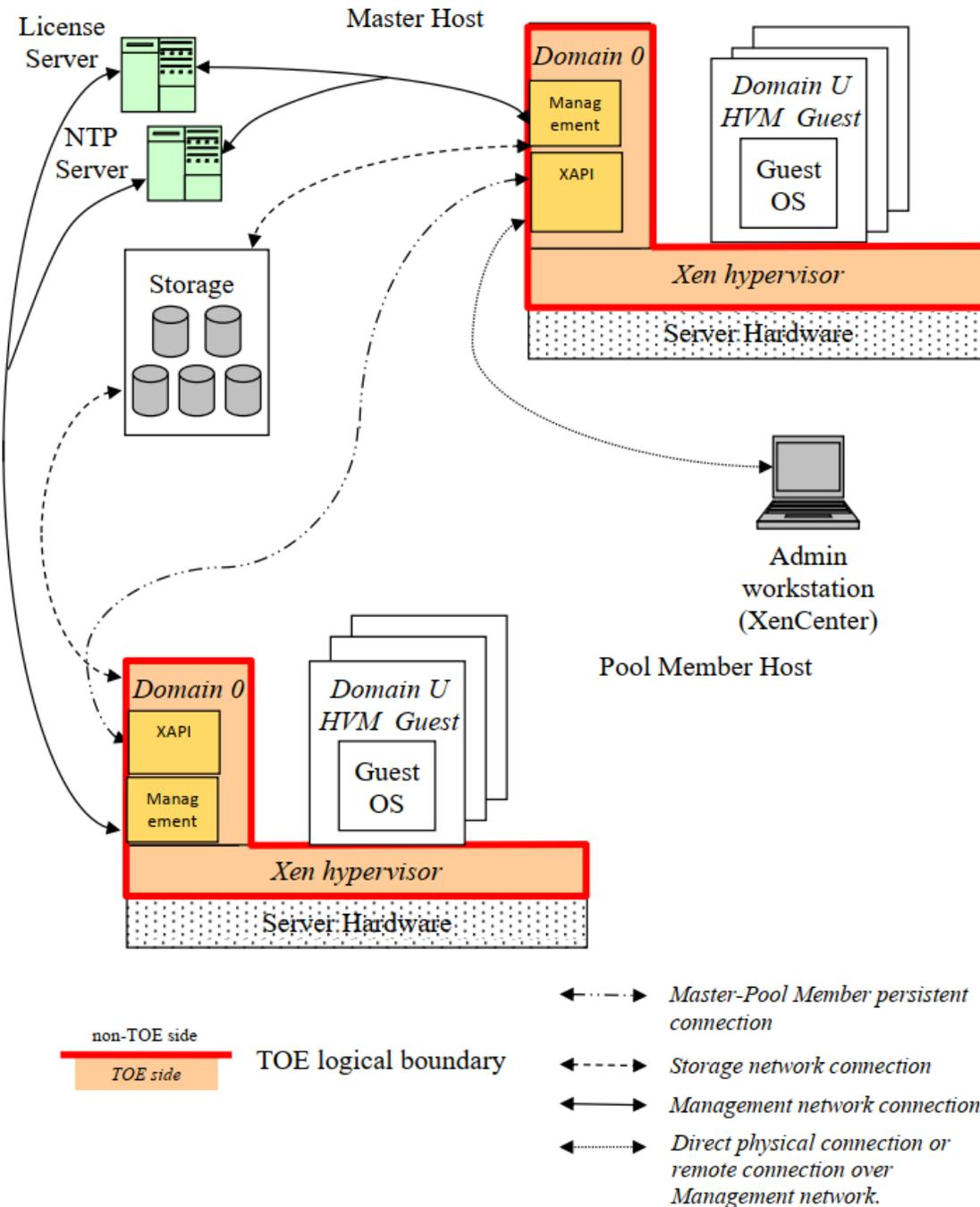
Figure 1: TOE Architecture
